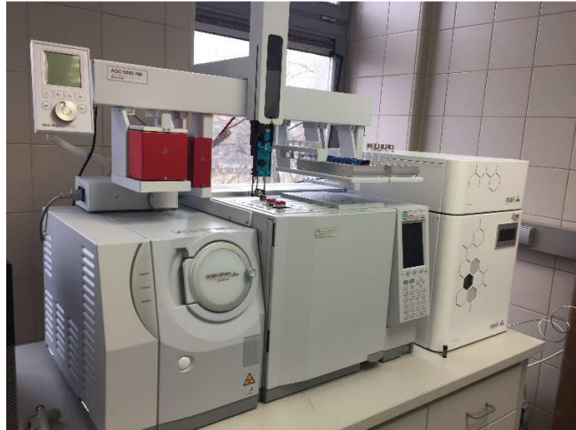
Gas chromatograph (Shimadzu) (GC) with mass (MS) and ion exchange detectors (FID), which has a static headspace for samples that contain high molecular weight
