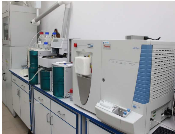
High pressure liquid chromatography (HPLC) system Varian ProStar (Varian Corp., USA) with UV/VIS Detector Varian ProStar 325 , Varian ProStar fluorescence detector 363 and mass spectrometer Thermo Scientific, LCQ Fleet .
